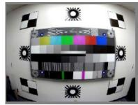
Even small vibration of the test chart will be interpreted by VQMA as increase of camera noise and drop-down of frequency response, so it is important to fix the chart firmly on something solid. Same applies to camera itself - any vibration during video data capture is highly undesirable. **Fluorescent light sources** are also undesirable. They produce **flickering light**, significantly biasing VQMA noise analysis results.
