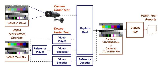
Test pattern video data should be stored on fast access media, e.g. HDD, in a media file(s), such as raw data YUV file(s) or wrapped YUV/RGB file(s) containing **single video frame** *or* at least **8 consecutive video frames** in **uncompressed** or **compressed** format.
