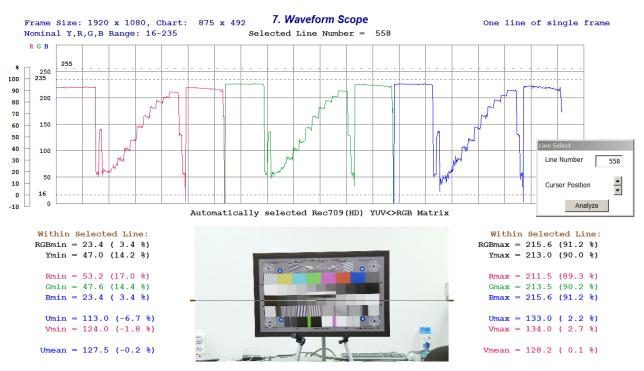
All YUV/RGB waveform diagrams are shown superimposed over the standard levels vs pixels grid.
