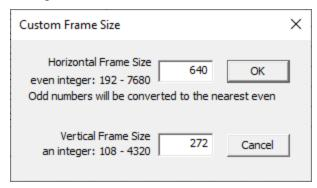
Clicking "Set Custom Frame Size" launches separate pop-up Dialog Box. It allows entering *even* integers for the *horizontal* size or *any* integer for the *vertical* size; in both cases the permitted ranges are *automatically clipped*. Note that the selected frame size should **exactly match** the . YUV file to be opened.
