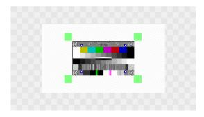
Note that **Vertical Chart Size** = **360** means danger of *aliasing artefacts* on bursts # 4, 5 and 6, i. e. incomplete suppression of 400, 500 and 600 tvl frequencies, exceeding 360 tvl limit.
