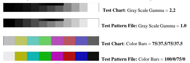
Because VQMA is a **mainly static** test pattern, video **frame rate** and **interlace ratio** do not affect the analysis results.
