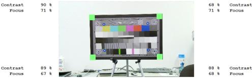
Green squares mark actual measured positions of the chart edges. They may exactly touch the frame corners, if scale is exactly 100%. Markers are inside the frame, if scale is less than 100%, or slightly outside of cropped chart image, e.g. for scale = 105%.
